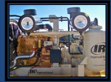
Diesel engine with electronic controls to comply with USA/EPA Tier 3 exhaust emission requirements. • Three stage, heavy duty, dry type air cleaner with replaceable primary and secondary elements located inside unit. Air filters have maintenance indicator lamp on the control panel. • Fuel/water separator.
